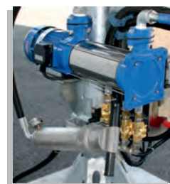
Pompa, valvole. Water distribution by solenoid valves and water filter installed on the A-60 industrial dust suppression fog cannon.
