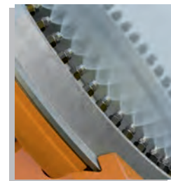
Anello ugelli. Apache A-60 industrial ventilator head view with detail of the three sectors single nozzle ring.
